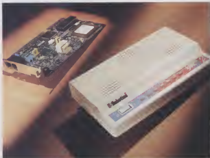
Life in the Fast Lane: Squeeze more modem performance from standard analog phone lines. The internal Diamond Multimedia SupraExpress 56i (left) and the external U.S. Robotics Sportster 56K Faxmodem (right) hit download speeds of 56Kbps.
